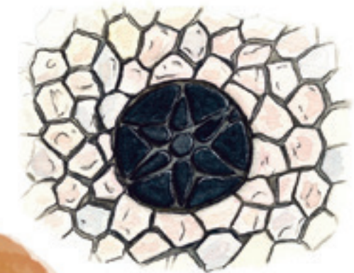
Portuguese pavement in limestone and basalt
